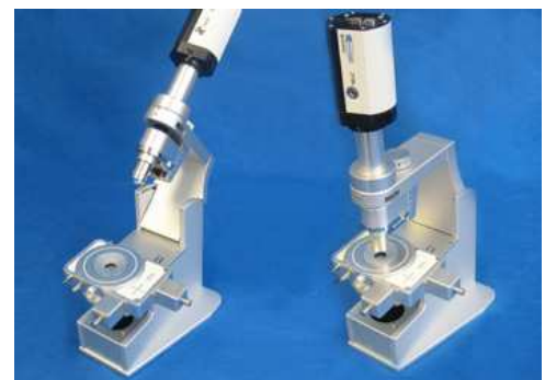
Linkam Imaging Station. Optics are tilted back to allow easy access to sample
