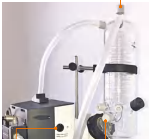
Opening for vapor temperature sensor Temperature sensor connection
