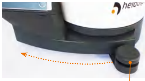
Handlift-Hebel: Liftposition oben
