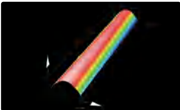
Corrosion on stainless steel / Height measurement (MPLAPON20XLEXT / 3 x 3 stitched)
