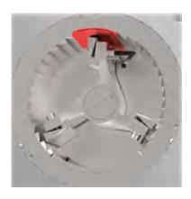
The impact plates experience a certain amount of wear during use. If there is a high degree of wear, the gap between the impact plates and grinding insert becomes too large. You can reset this gap with the help of the supplied setting plate.
