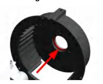
Grease the felt ring (F) in the grinding chamber cartridge every week with a few drops of machine oil.
