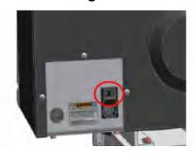
■ Ensure that the mill is closed before switching on the device using the main switch on the reverse. (I)
