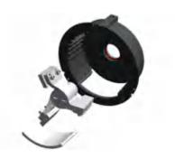
To facilitate cleaning, the grinding chamber, bottom sieve and cross beater can all be removed. For this, see Chapter & Chapter 6.3 'Installing the grinding elements' on page 24.
