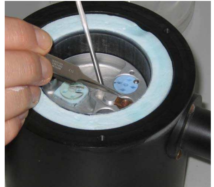
Load the frozen hydrated specimen into the cryo-transfer holder
