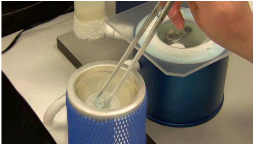
Transfer frozen hydrated specimen from the workstation of Cryoplunge 3 system
