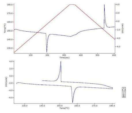
The graphs shown are typical DSC curve outputs from the LINK control software; indium samples are on the left and copper sulphate on the right.
