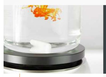
Hotplates made of aluminum guarantee the fastest heat-up times. However, they are not chemical-resistant or scratch-resistant.
