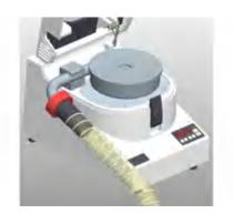
**3.** Slide the rubber sleeve with the exhaust hose from the cyclone separator over the outlet of the grinding vessel.
