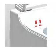
**2.** Remove the cover screws in the lower part of the housing.
