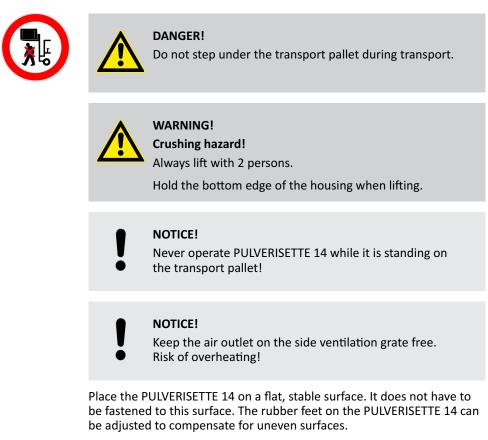
Make sure that the PULVERISETTE 14 is easily accessible. There has to be sufficient space to reach the main switch on the back of the device.
