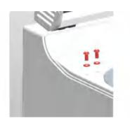
**2.** Remove the cover screws in the lower part of the housing.
