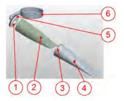
**4.** Insert the paper filter sack (2) in the nylon support sack (4) and clamp it firmly at the plastic flange (1) with the clamping ring (3). Make sure that the nylon support sack has been slid over the rubber seal (5).
