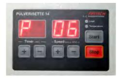
When the mill is switched on, the values of the last milling are displayed.
