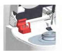
**3.** Fasten the bent tube support there.
