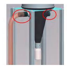
**4.** Fasten the other end of the exhaust hose on the open hose connecting tube of the cyclone separator.
