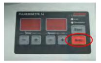
**1.** When the device has been switched off, press and hold the STOP button on the front control panel.
