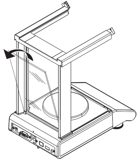
9 Remove weighing pan, pan support and bottom plate.
