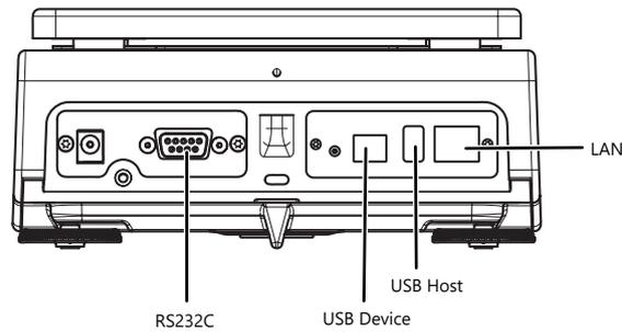
Interfaces and possible connectivity of peripheral devices:
