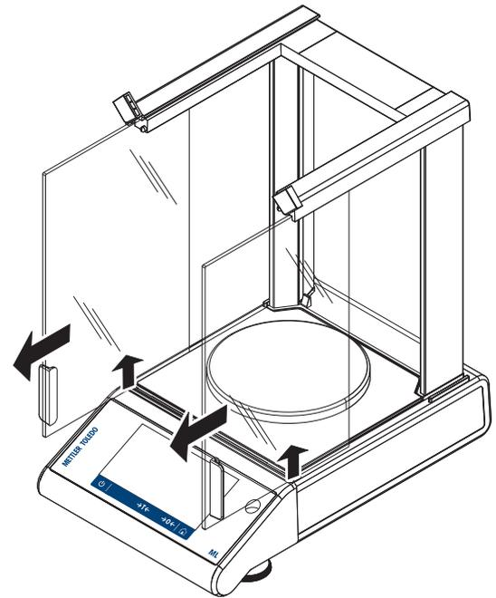
7 Push the lock button to release the rear glass.
