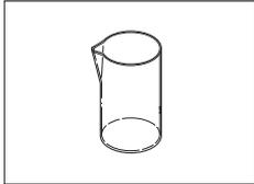
Glass beaker, height 100 mm,  $\varnothing$  60 mm
