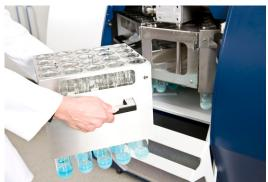
Kjeltec™ 8400 is a fully automated Kjeldahl analyser with self-cleaning colorimetric titration and optional auto samplers for fully unattended operation of up to 60 samples. Take your protein and nitrogen analysis to new levels of efficiency with renowned accuracy, cost effectiveness and safety.
