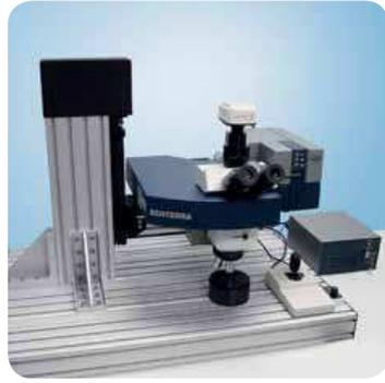
SENTERRA configured as an open architecture microscope.
