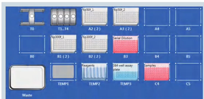
Figure 2: Screenshot of the worktable layout for the file Thrombin_inhibition.
