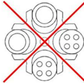
Fig. 5: Permissible and impermissible loading of a swing-out rotor with different tube sizes (example illustration)
