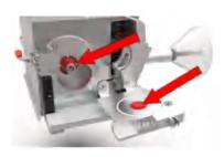
**4.** Clean both cone-shaped holders (cones) in the closing lid (3) and on the holder.
