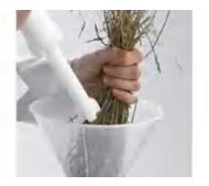
The plunger has 2 different sides for feeding the sample material in the funnel to the grinding chamber. On the one hand, the smooth, round side is suitable for finer material. On the other hand, the cross-shaped, thinner side is suitable for long, fibrous material, like straw.
