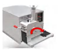
Insert the provided hexagon socket screw key through the central bore hole. Then turn the hexagon socket screw key to check if the rotor (10) is turning freely.
