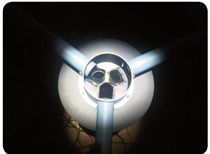
Fig. 3: Close view onto the 3 \times 120^\circ reflective beam splitter that evenly distributes the IR radiation to the input ports of the IFS 125HR spectrometers.
