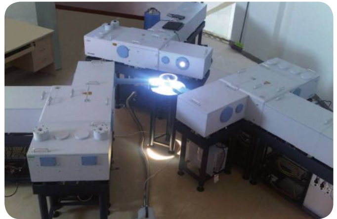
Fig. 2: Arrangement of three compact IFS 125HR spectrometers installed in the new astronomical observatory at the Shenzhen Meteorological Bureau in China.
