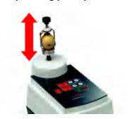
The rapid vertical acceleration of the grinding bowl causes the grinding balls in the bowl to vibrate. Comminution occurs when the balls of grinding stock hit the walls of the bowl and each other. Due to the almost spherical grinding chamber the balls are not limited to vertical movement, and very efficient comminution is achieved.
