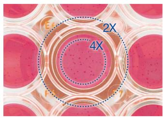
When viewing a 96-well plate, the wide visual field allows all the cells in a well to be observed without moving the stage.
