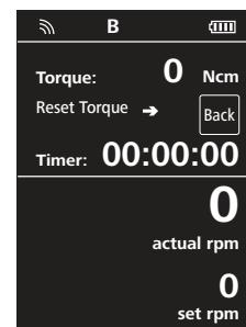
Rotate the rotary/push knob (**B**, see **Fig. 1**) to set the target speed. Press the rotary/push knob (**B**), the stirrer starts to run with the set speed.
