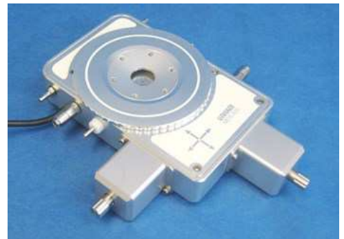
The MDSG600 heating and freezing stage
