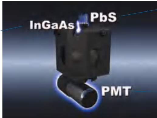
Three detectors attached to the integrating sphere
