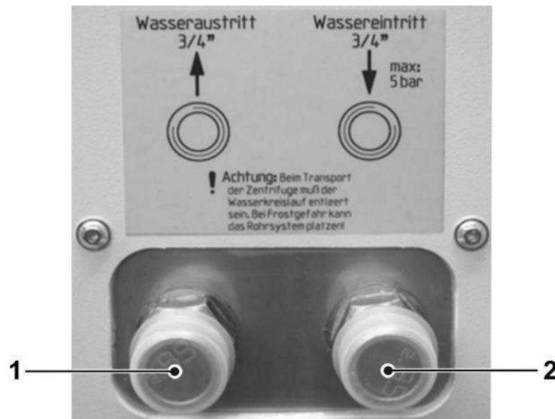
Fig. 8: Connections for the cooling water system
