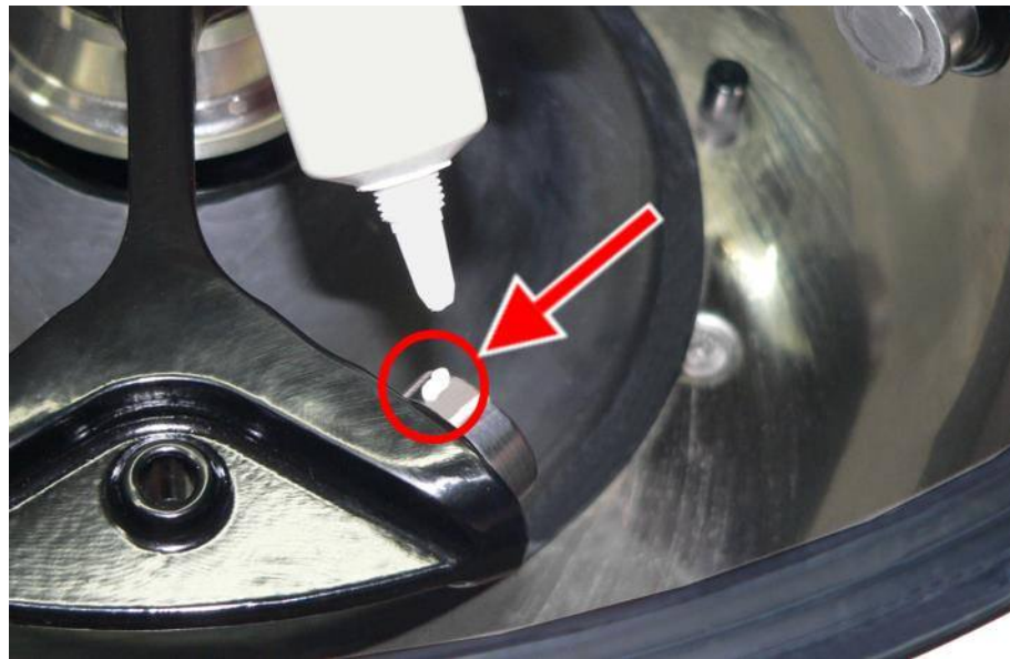
Fig. 36: Sufficient quantity of grease for one bolt
