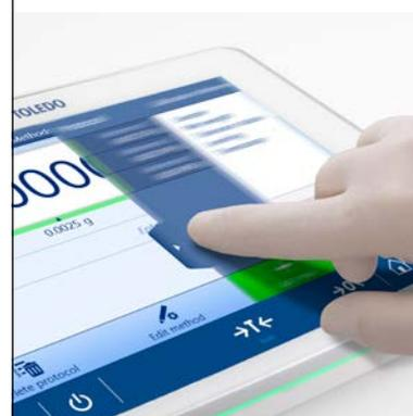
The new capacitive touchscreen enables you to 'swipe' through your tasks as well as use multiple fingers to type in data. The screen is operable even through thick chemically resistant gloves, such as those in glove boxes.
