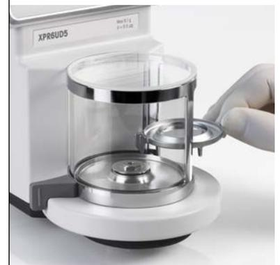
The newly designed draft shield provides easy access to the weighing pan. There are no edges and corners where sample material could become trapped. All parts can be removed, cleaned and replaced in a few simple steps.
