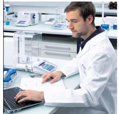
Balance calibration is at the core of accurate weighing results. Each calibration certificate declares the balance's minimum weight and measurement uncertainty – essential information for reliable weighing processes.
