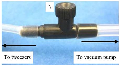
Use a finger to block the hole of the tweezers to pick up a sample cover slip with the suction cup.
