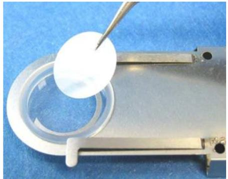
Before loading the Crucible Carrier the silver block must be prepared with silicon oil to provide a good thermal contact between the crucible and the silver block when the stage is under a vacuum.
