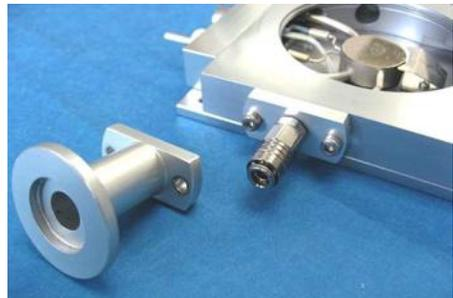
The Gas Connector is self closing, it is open when the Gas Insert is pushed into the Gas Connector.
