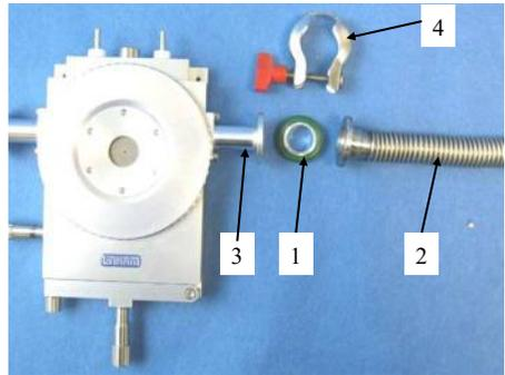
Ensure that the O-ring is correctly seated in the Steel Vacuum Tube and vacuum connector before tightening the Clamping Bracket (4) screw (5).
