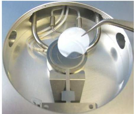
Using a pair of tweezers place a Shim Spacer (1) in the middle of the Sample Holder.
