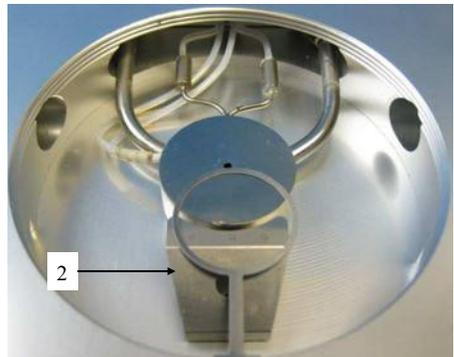
At standard atmospheric pressure the contact between the sample and the silver block is enough to establish good thermal contact as the air molecules in any minute scratches will conduct the heat, but when pulling a vacuum these are drawn out of the stage. Objective immersion oil (supplied) has the same refractive index as quartz and ensures an almost perfect thermal seal between block and crucible.
