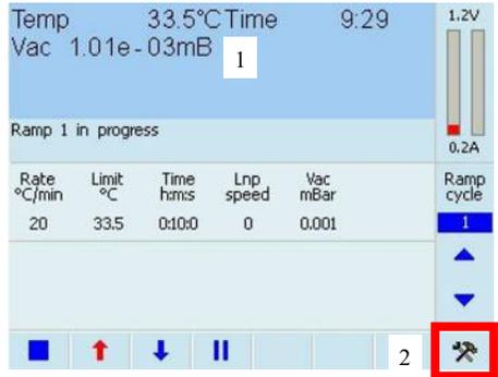
To change the vacuum unit, touch the Setup icon (2) to go to the Setup Tab page.
