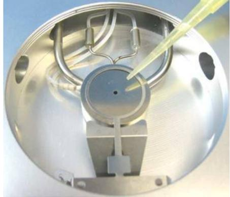
Use the supplied Vacuum Tweezers or a pair of tweezers place a clean W16Q, (16 x 0.3mm) Quartz Sample Window directly on top of the oil inside the G16.3 Sampler Holder.
