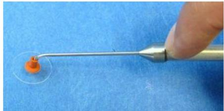
Release the finger to drop the sample cover slip.
