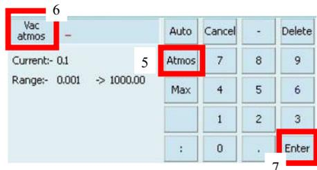
3. Max: in this mode the motorised valve will close fully to get the maximum vacuum from the vacuum pump.
