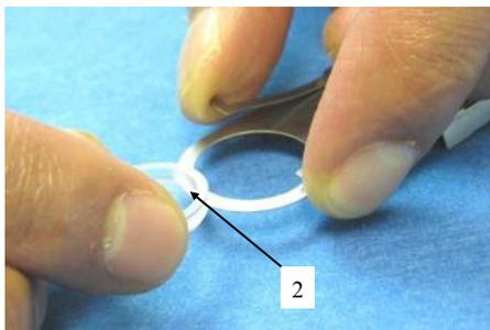
Release the two spring clips to hold the Crucible in place.
