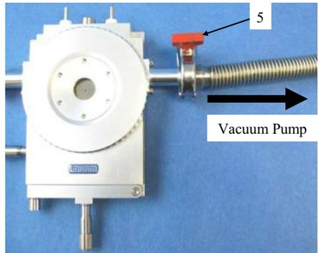
Note: the FDCS196 is only tested with a vacuum of  $10^{-3}$  mBar. Do not use a vacuum lower than this.
