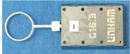
To load the G16.3 into the FDCS stage, open the door of the stage by unscrewing the door thumbscrew. The G16.3 slides into the brass housing located just inside the door.
