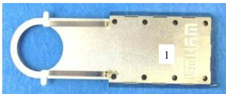
To load the quartz crucible into the carrier, lift the two spring clips about 2mm upward and slide the crucible in to the holder.
