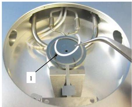
Pipette 2 $\mu$ l of sample on the Quartz Sample Window inside the Shim Spacer.
