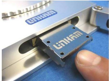
The Sample Holder Ramp (2) will guide the G16.3 up on to the silver block.
