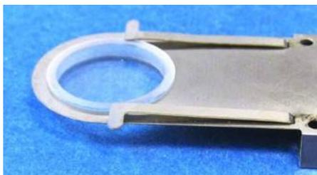
Use a pair of tweezers to place a Shim Spacer inside the Quartz Crucible.
