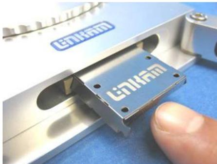
With one hand push the FDSC/CC and with the other hand lift the edge of the crucible up the ramp and over the drop of oil. When the drop of oil is roughly in the centre of the crucible gently lower the crucible on the block. Now close the door of the stage and screw in the door locking screw. This screw only needs to be finger tight.
