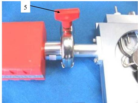
Connect the Pirani Cable with the LAN type connector (5) to the Pirani and the other end of the cable to the back of the T95; Slot 4; labelled 'VAC', see page 9.
