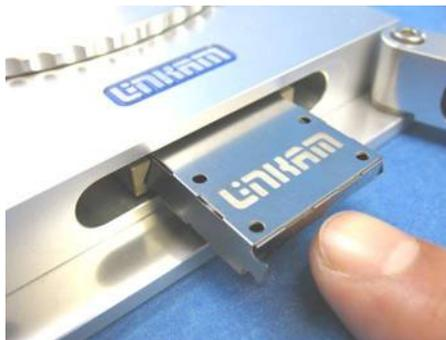
The crucible will be guided to the surface of the silver block by the Sample Holder Ramp. Close the door and tighten the thumbscrew to seal the stage.
