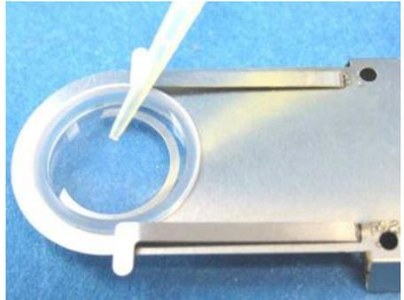
Use the supplied Vacuum Tweezers or a pair of tweezers to place a clean W13G, (13 x 0.17mm) Glass Sample Window on top of the sample, ensure it touches the Shim Spacer.
