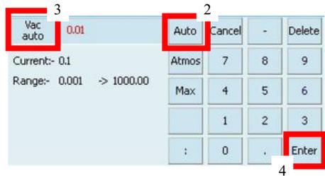
Note: The MV196 is only designed to hold a controlled vacuum between **100mbar to 0.1mbar**. Any values outside this range may not be accurate.
