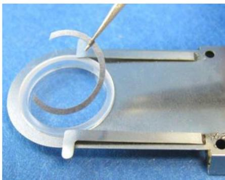
Pipette 2 $\mu$ l of sample inside the Shim Spacer.
