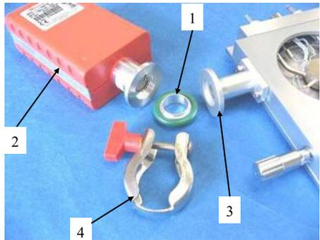
Ensure that the O-ring is correctly seated in the gauge and vacuum connector before tightening the Clamping Bracket (4) screw (5).
