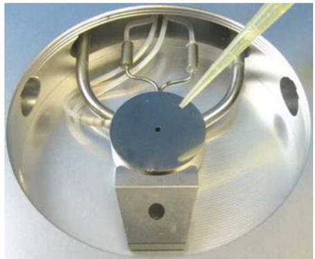
Load the Crucible Holder with the prepared sample into the FDSC196 stage. Unscrew the Y manipulator (the one screwed into the stage door) so that when you close the door, the FDSC/CC doesn't push the crucible right off the edge of the block and the silicon oil with it.
