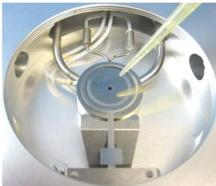
Use the supplied Vacuum Tweezers or a pair of tweezers place a clean W13G, (13 x 0.17mm) Glass Sample Window on top of the sample, ensuring it touches the Shim Spacer.
