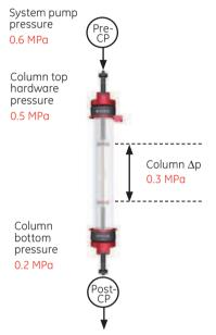
Fig 5. For increased operational safety, the column selection valve enables continuous measurement of precolumn (Pre-CP) and post-column pressure (Post-CP) during runs. The pressure difference over the packed media bed  $(\Delta p)$  is calculated from the two signals.
