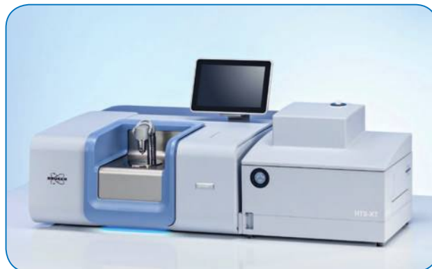
Figure 11: HTS-XT high throughput accessory with INVENIO S spectrometer.
