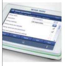
Titration Excellence instruments are equipped with a comprehensive user management system that allows you to register each user and to set up a Homescreen for each user. Depending on who logs on to the titrator, the corresponding Shortcuts together with the other user-defined settings appear such as screen settings or the language the user requires.
