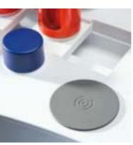
A SmartSample reader is installed as standard on all Excellence instruments. Wireless data transfer from balance to titrator is now possible on single samples, eliminating transcription errors due to manual entry. The SmartSample solution is therefore an intelligent choice for both single- and automated multi-sample titration.
