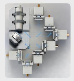
Each PMT is placed an equal distance from the flow cell so optimal light can be achieved at all wavelengths without compromise.
