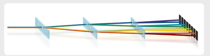
An optical filter layout with consistent path lengths yields optimal detection and sensitivity for all wavelengths at each detector.
