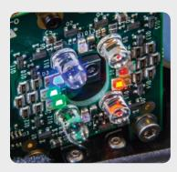
A series of LEDs of different wavelengths illuminate the light path. The amount of light reaching each PMT from the different wavelength LEDs is determined by the filters that are in place. The detected PMT signal is compared to a reference to determine whether the expected filter set is in place. If the signals do not match, a warning will be displayed at the relevant PMT(s).
