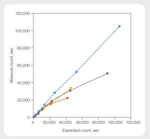
This graph shows the acquisition speed capabilities of the ZE5. Dragon Green Beads (Bangs Laboratories, Inc.) were used in a serial dilution to determine when the observed acquisition rate falls off the theoretical limit. The ZE5 outperforms other systems at higher acquisition speeds as it continues to acquire data into the 100,000 events per second range whereas the other systems fall off around 20,000 events per second. ZE5 Cell Analyzer (—); Cytometer 1 (—); Cytometer 2 (—); Cytometer 3 (—).
