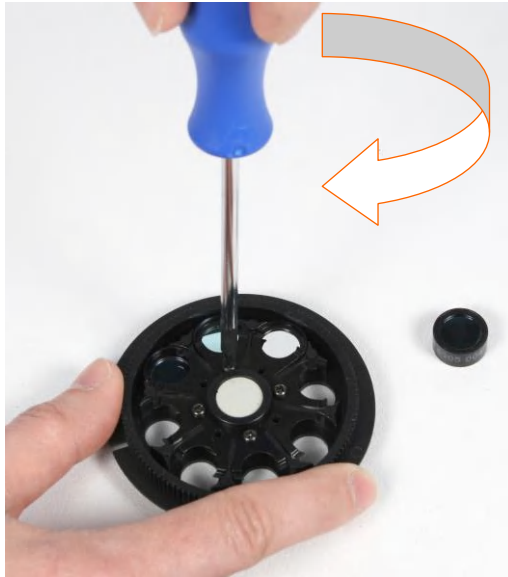
Figure 20. Removing the spring position holding screws
