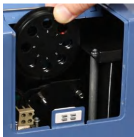
Figure 8. Placing the Multiskan FC filter wheel into the filter slot
