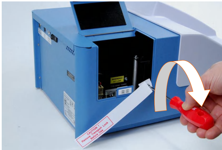
Figure 28. Fastening the transport lock
