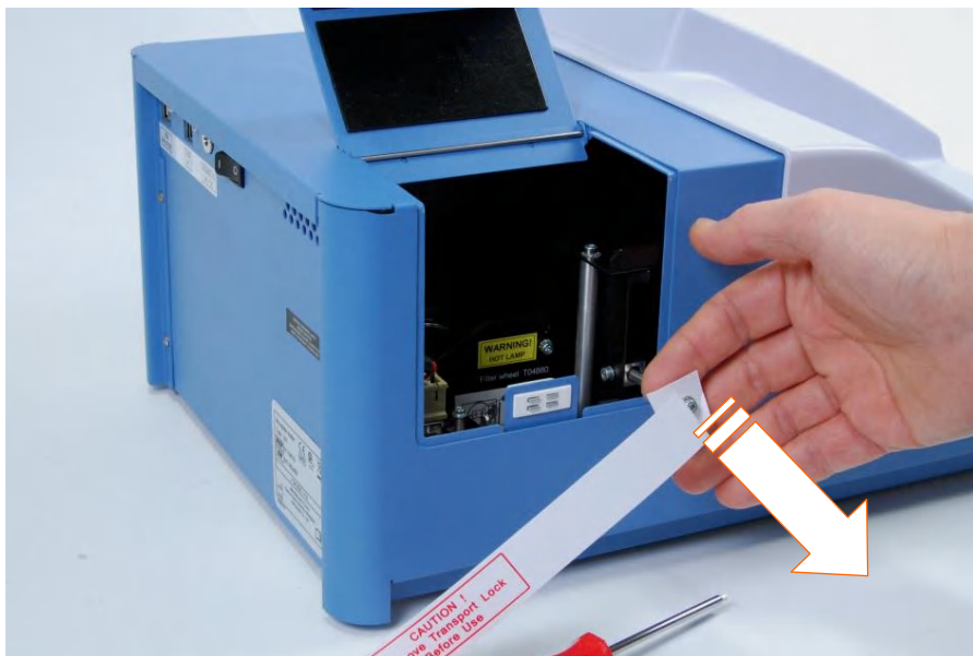
Figure 5. Pulling the transport lock out
