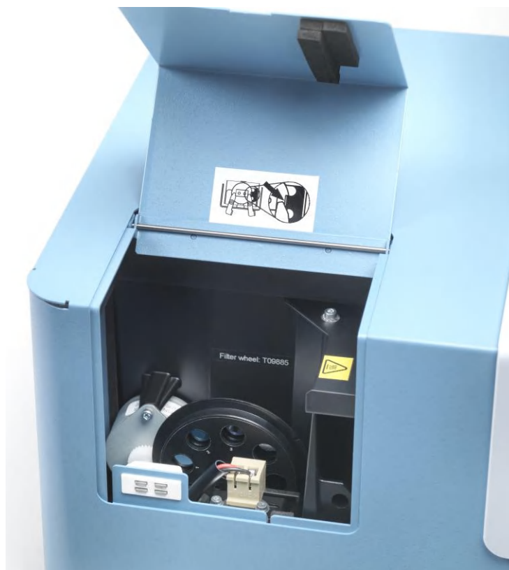
Figure 19. Removing the filter wheel
