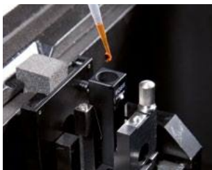
Adjustable cell holder with ultra-micro cell for extremely small sample volumes
