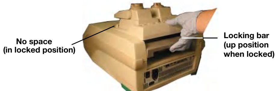
Figure 5. Locking the reaction module in place.
