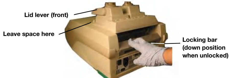
Figure 4. Inserting the reaction module into the bay.
