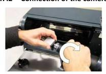
**1.** Remove the caps from the camera and from the screw thread of the lens. Screw the lens hand-tight onto the camera!
