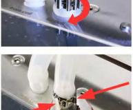
Before replacing the hoses, the measuring liquid must be drained from the system. To do this empty the system as described in Chapter \$ Chapter 7.6.3 "Emptying the system" on page 52.
