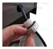
**4.** Press the threaded cable gland (4) together and guide the seal ring over the thread.
