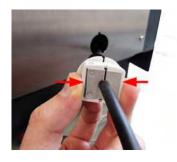
On the back of the ANALYSETTE 28 ImageSizer, insert the seal ring and then slip the threaded cable gland (4) over the cable.
