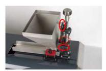
**7.** Re-tighten the clamp screws.
