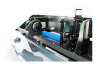
Insert the camera with lens. To do this, hold the lens tilted backwards in the device housing, as shown in the picture, and hook the flat rail runner onto the rail from behind. Then tilt the lens forwards and position it on the rail. The lens holder can be moved back and forth on the rail.
