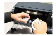
6. Now, as described in ♥ Chapter 4.7.2 "Connection of the camera to the lens and insertion" on page 26, connect the other lens to the camera and place it in the device.
