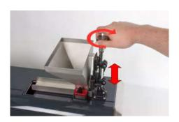
Turn the knurled screw on the top of the funnel support column in order to move the funnel up and down.
