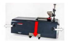
Open the front flap (7) forwards by lifting up both latches (6).
