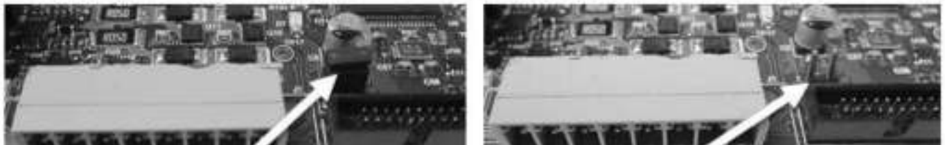
Figure 6-7. Jumper Cap for Hysteresis & Dual Probe Fault Mode Selection
