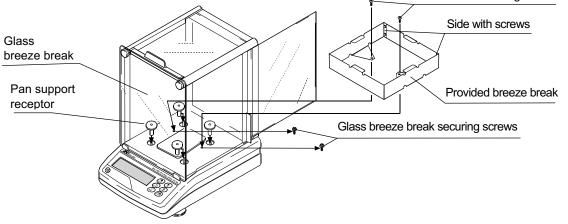
2. Place the auto-centering pan guide on the pan support receptors, and then place the auto-centering pan on the guide.
