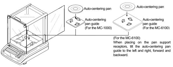
Note: When replacing the weighing pan with the auto-centering pan, be sure to calibrate the balance before weighing, because the two pans are different in weight.
