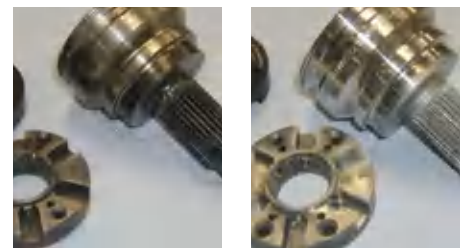
Removal of oxidation and other contaminants
