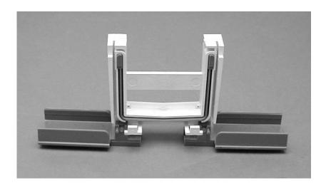
b. Place gel sandwich or gel cassette into the clamping frame with the Mini-PROTEAN 3 short plates facing inward. Note: the clamping frame requires 2 gels to create the clamp assembly. If an odd number of gels are being run, use the buffer dam.
