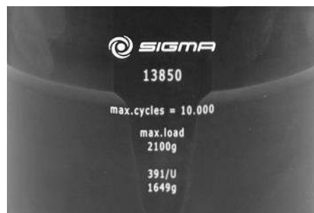
Fig. 4: Different service life – engraving on the bucket/rotor
