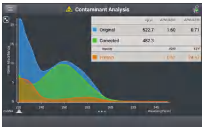
dsDNA sample contaminated with protein. The absorbance contribution from the protein (orange) is subtracted from the original result (blue) to obtain the corrected dsDNA concentration (green).
