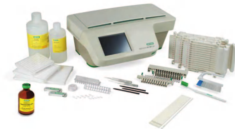
Fig. 1.1. PROTEAN i12 IEF system. The system includes the PROTEAN i12 IEF cell and numerous accessories.
