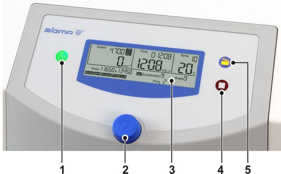
Fig. 9: User interface of the Spincontrol L control system
