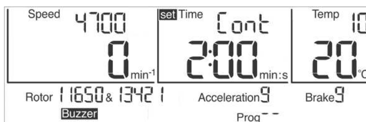
Fig. 14: Indication "Cont" during a continuous run
