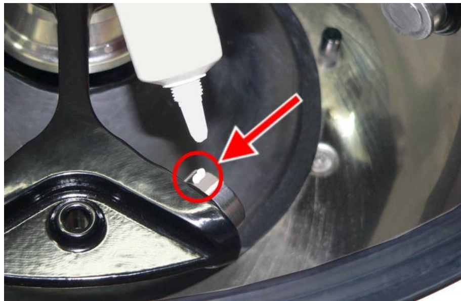
Fig. 29: Sufficient quantity of grease for one bolt
