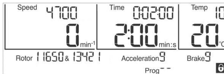
Fig. 25: "Padlock" symbol indicating an activated input lock
