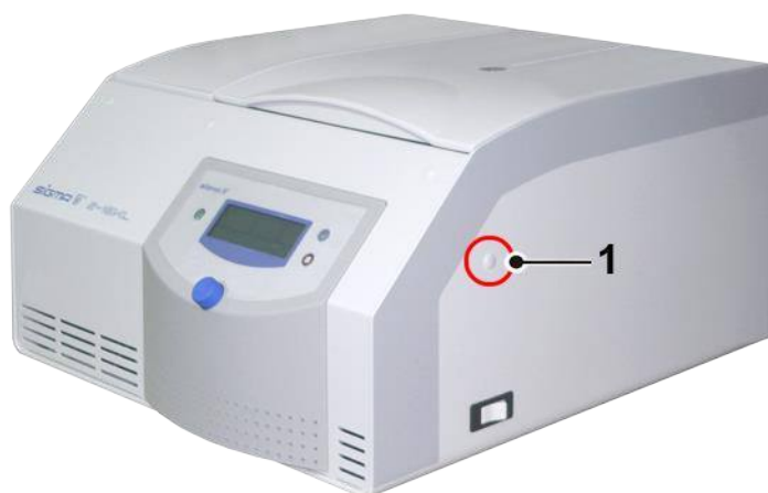
Fig. 28: Position of the opening for the emergency lid release
