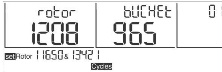
Fig. 23: Cycle display for rotor 11650 and bucket 13421
