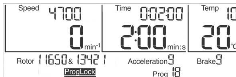
Fig. 22: The program lock "ProgLock" is activated
