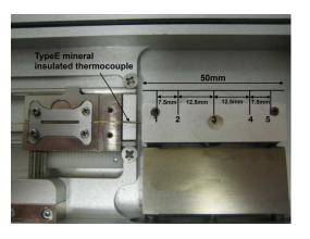
CAP500 Stage temperature difference along heater
