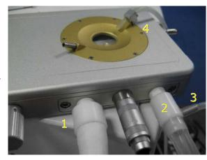
The short tube branching from the side of this white connector is the Gas Purging Tube (3).
