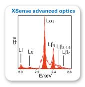
Molybdenum spectra obtained with standard (outline) and advanced optical system (solid).
