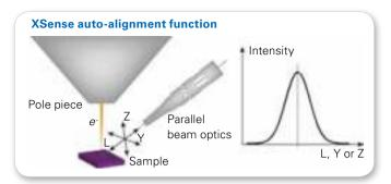
XSense can position the spectrometer optics along 3 axes for perfect automatic alignment.
