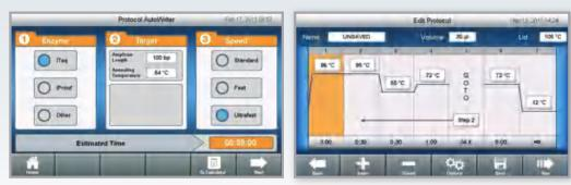
Quick and easy protocol programming. The protocol autowriter in the cycler's onboard software can automatically suggest a fast temperature protocol based on input parameters. Suggested protocol is based on standard PCR guidelines, with hot-start, initial denaturation, annealing, and extension steps. Further reductions of run times are achieved by minimizing the number of steps and cycles, incubation times, and temperature differentials.
