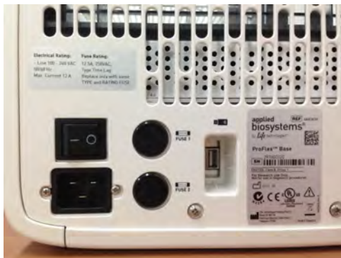
Figure 39 Location of the safety label on the rear panel of the ProFlex™ Thermal Cycler
