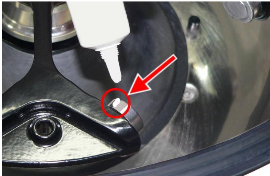
Fig. 32: Sufficient quantity of grease for one bolt
