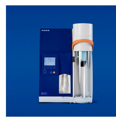
Kjeltec<sup>™</sup> 8100 is a semi-automated distillation unit designed primarily for Kjeldahl analysis, but widely used for many different distillation chemistries.
