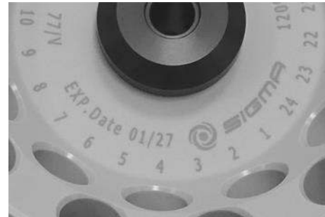
Fig. 4: Different service life – engraving on the bucket/rotor
