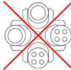
Fig. 7: Permissible and impermissible loading of a swing-out rotor with vessels of various sizes (example illustration)
