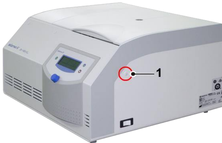
Fig. 29: Position of the opening for the emergency lid release
