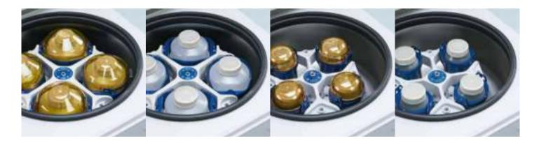
New large volume bottles in Centrifuge 5910 R: 1,000 mL bottles in Rotor S-4xUniversal (left) and 400 mL bottles in Rotor S-4x400 (right) with and without aerosol-tight caps for safe centrifugation of hazardous samples.
