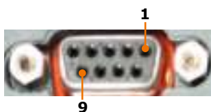
SUB D9 plug Device connection
