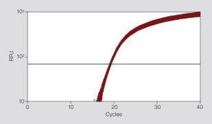
**Excellent uniformity.** *IL-1β* plasmid template diluted to  $10^{\circ}$  copies/reaction amplified in the presence of a FAM dye–labeled detection probe with iQ Supermix. Graph shows 96 replicates of 10 µl reactions. Average quantification cycle (Cq) =  $19.81 \pm 0.10$ . RFU, relative fluorescence units.
