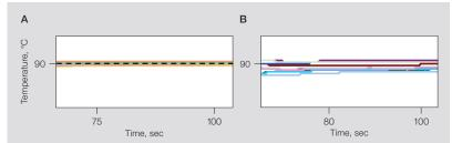
Superior thermal uniformity for reproducible results. The temperature measured by probes in 15 wells across a sample block. A, temperatures across the sample block vary by  $\pm 0.3^{\circ}$ C for the CFX Opus Systems, an improvement of 0.1°C over B, the temperature variability across the CFX Touch Systems' sample block.
