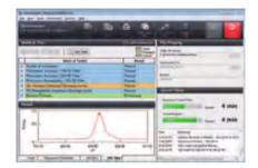
The user can select confirmation of instrument performance indicators as per JIS K0115 General rules for molecular absorptiometric analysis, as well as the general test methods in the Japanese Pharmacopeia, USP and various EP inspections. (Order inspection jigs and reagents separately.)
